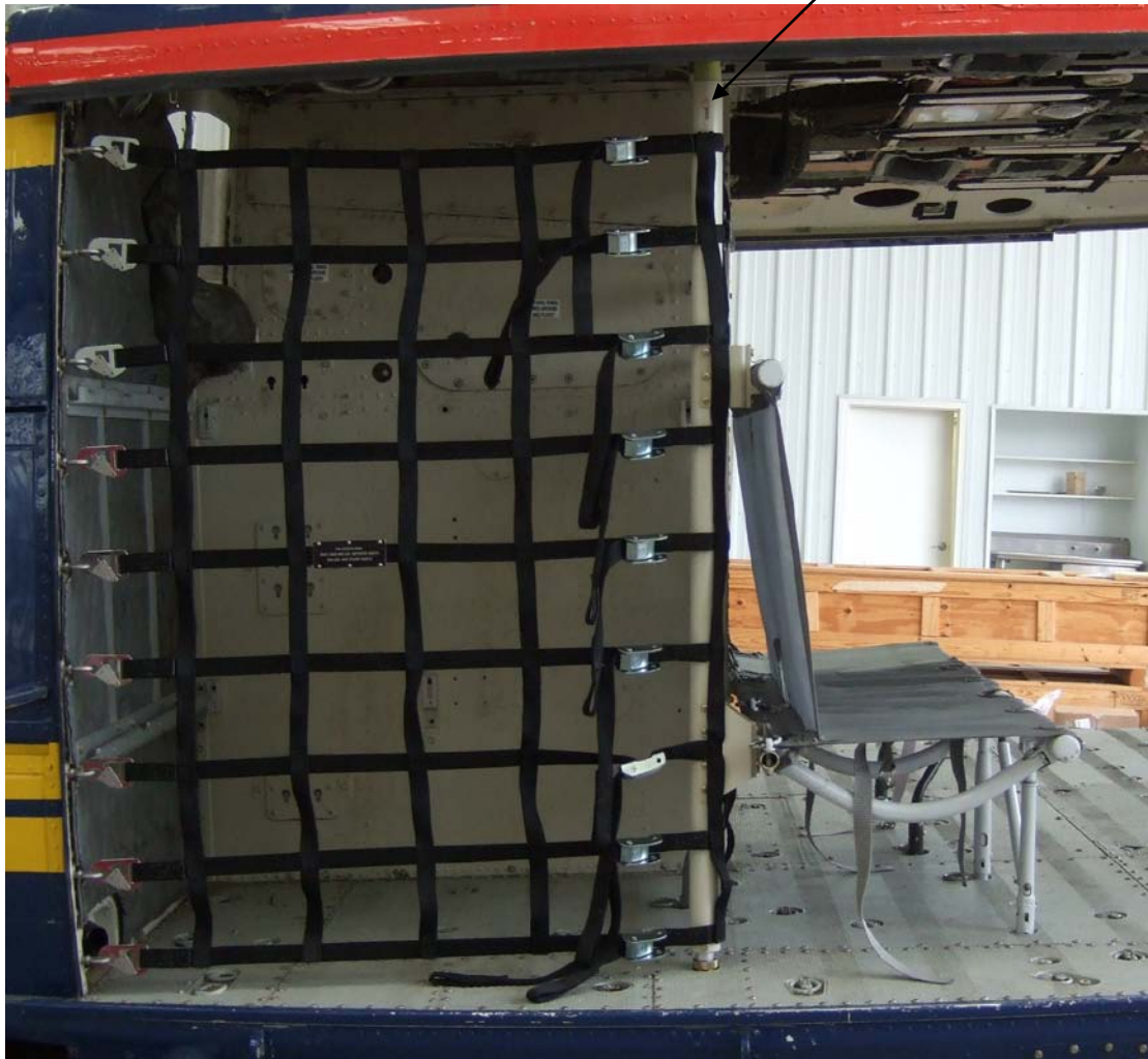
Figure 11 Support Pole (P/N 2550-02-0001) Installed with Adjustable Adaptor Up
